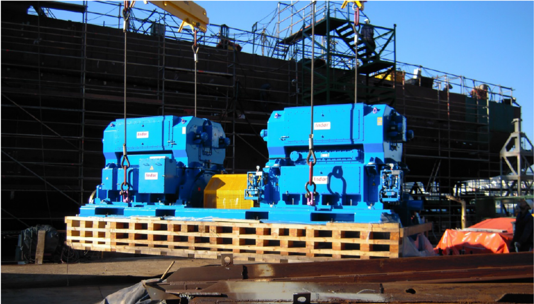
AC motors prepared for on board installation - 01.10.15
